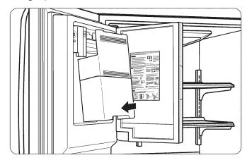
4. Avoid touching the automatic shutoff arm when replacing the ice bank. See the label on the ice bank door for details.
